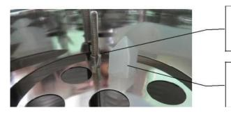
Wing nuts to secure compression plate
